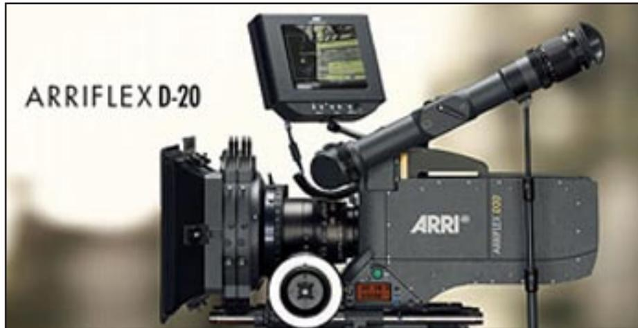
The ARRIFLEX D-20 is a film style digital camera. Because of its single, Super 35-sized CMOS sensor, the D-20 uses the same lenses as 35mm film cameras and has the same depth of field as 35mm film. It has an optical viewfinder, is capable of variable frame rates and is compatible with ARRI film camera accessories. It outputs an HDTV signal in HD mode or via raw sensor information in data mode. See [www.arri.com](http://www.arri.com).
